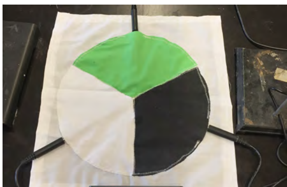
Figure 1 – Albedo lab apparatus with the LabQuest 2, this also works well with alcohol thermometers.
